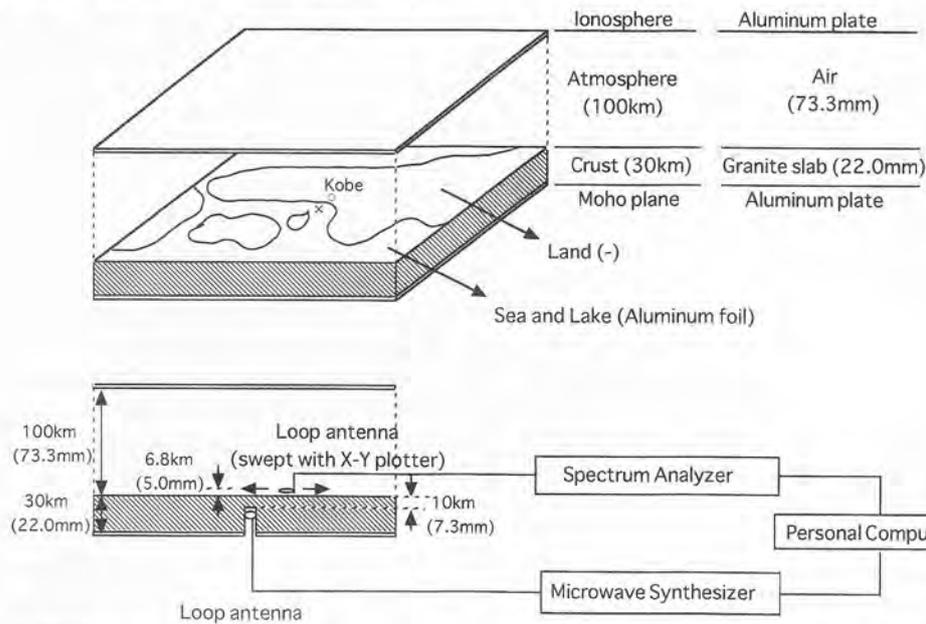
Fig. 1. A schematic drawing of the Japanese island archipelago model simulating the ionosphere, the Earth surface and Moho plane using aluminum plates and foil and a 22 mm thick granite slab. Electromagnetic waves were emitted from a small antenna below the slab surface and detected using another antenna 5 mm above the surface.
