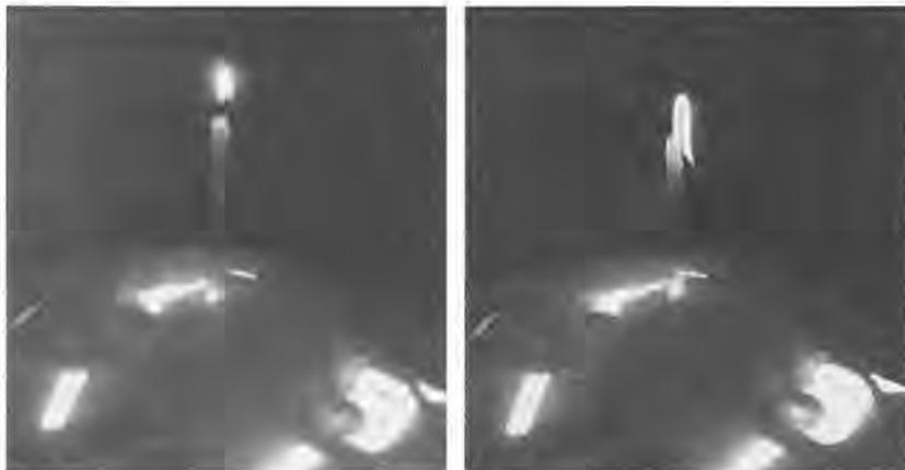
Fig. 1a,b. Bending of a candle flame before a temple or shrine altar as a precursor of an earthquake is a proverb in Japan. This is reproduced in an electrostatic experiment. a) A candle flame on electrically grounded sphere of a Van de Graaff electrostatic generator. b) The same candle after the sphere was charged to give 250 kV
