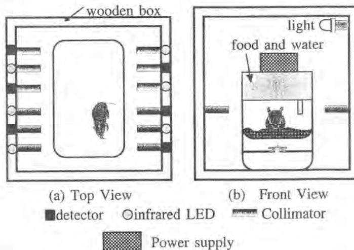
Fig. 3: Mouse activity monitoring system of (a) top view and (b) front view. The locations of detectors and infrared LEDs are shown. Electromagnetic pulses were generated in the down-side box. The power supply was placed on the top.
