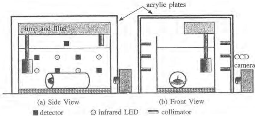
Fig. 2: Sensor locations of (a) side view and (b) front view for automatic observation of catfish behavior. The CCD camera photographed the behavior but stored the data in a PC only when there is a movement.
